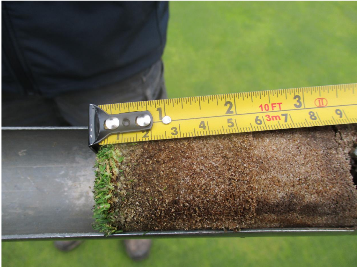
Sample from the 11th green showing the dense layer of organic material approximately 30mm in thickness.
