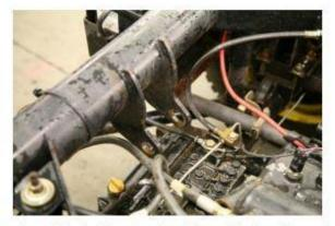
4. Rotate the hydraulic cylinder though 180°. Do not disconnect pipes.
