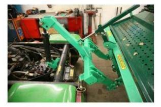
6. Attach Multi-Mount to Pro Gator as shown and connect the hydraulic cylinder.
