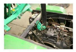
5. Refit hydraulic cylinder as shown.
