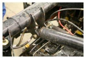
1. Dismount the tipping box, then remove the pin from the base of the hydraulic cylinder.
