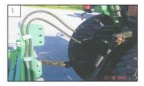
Fit the tractor lifting arms to the lower linkage pins of the Multi-Brush and secure with the lynch pins.
