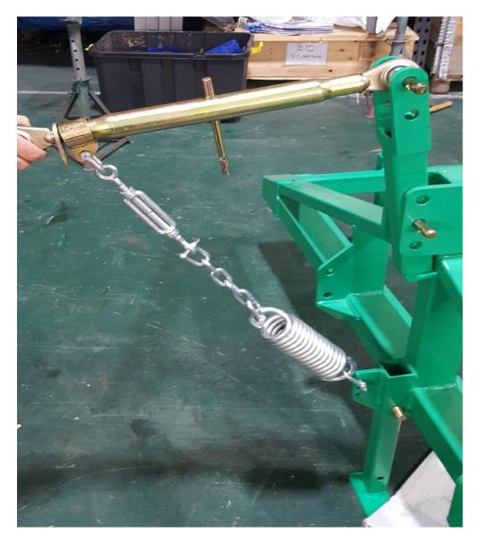
For use on golf courses where the direction of brushing involves traversing <u>across</u> severe ridge and furrow undulations, the optional Floating Top-Link Bracket shown above should be installed.
