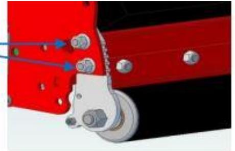
The rear scraper can be removed or simply be tied up. Use a ty-rop or rope and pull the scraper up. If the core collector is too aggressive, put an elastic band in the centre, which takes some weight off. In case the core collector hit the rear wheel, move the complete head forward, or remove the scraper completely.
