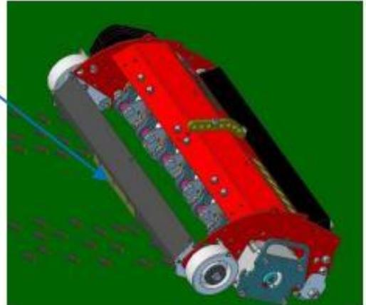
In case the full scraper isn't cleaning the surface well enough, an additional weight (a simple metal strip) can be mounted on the floating scraper base plate.
