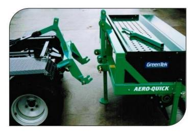
Fitting of top link extension post to Aero-Quick and adaptor frame to cushman
