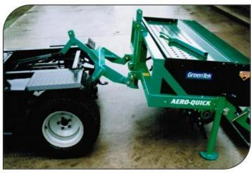
Adaptor frame raises Aero-Quick by its bottom link pins, allowing front stand leg to be raised.
